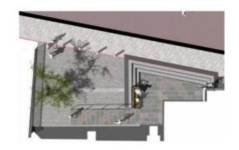
A new waterproof concrete floor slab has been laid in the North Porch, and onto this a new inclined stone and ceramic tile floor will be formed removing the current step.
